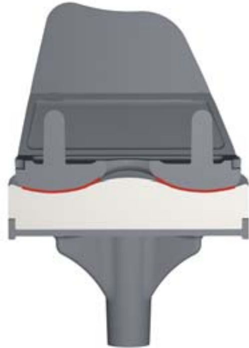
Figure 24: Optimized congruence between the femur and PE shown in the frontal plane.
